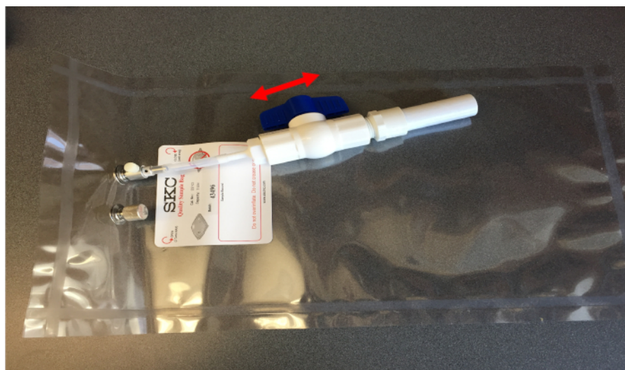
Figure 1: Assembled breath sampler and bag for exhaled breath collection. Breath sampler (with blue valve open, i.e., parallel with the connector as indicated by the double-sided red arrow) and bag connected with tubing, ready for breath collection. Please click here to view a larger version of this figure.
