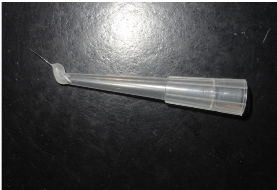
Figure 2: An example of a probe, fashioned with heat, from a pipette tip and a minuten nadeln pin. Please click here to view a larger version of this figure.
