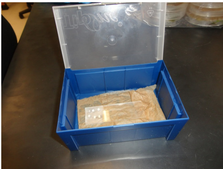
Figure 3: An example of a humidity chamber, fashioned from an empty pipette tip box and a wet paper towel. Please click here to view a larger version of this figure.
