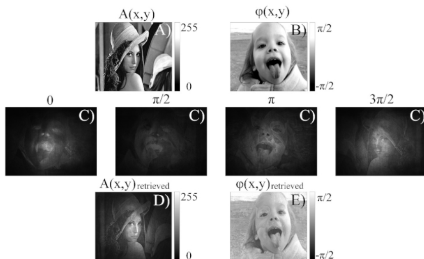
Figure 4: Representative experimental results under ultrashort pulsed illumination. (A) User-defined amplitude pattern of the complex field. (B) User-defined phase pattern of the complex field. (C) Interferograms associated with the polarization-based phase shifting technique developed in four steps and obtained after adding 0, \pi/2 , \pi , and 3\pi/2 to the phase element \alpha(x,y) . (D) Retrieved experimental amplitude pattern. (E) Retrieved experimental phase pattern. Please click here to view a larger version of this figure.
