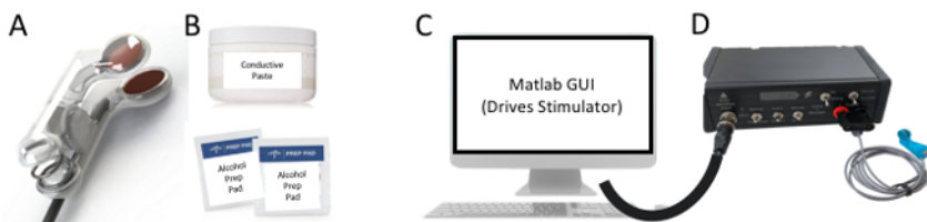
Figure 3: Key Components. The minimum required components for proper administration of taVNS are the following (A) ear stimulation electrodes, (B) conductive gel and alcohol prep pads, (C) computer capable of sending and receiving TTL pulses to a (D) constant current stimulator to trigger stimulation. Please click here to view a larger version of this figure.
