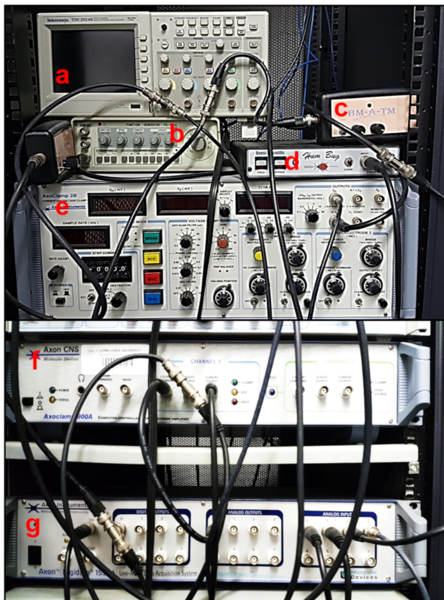
Figure 4: Equipment for running electrophysiology and data recording. a = oscilloscope, b = function generator, c = audible baseline monitor, d = 50/60 Hz noise filter, e and f = electrometers, g = data acquisition system. Please click here to view a larger version of this figure.
