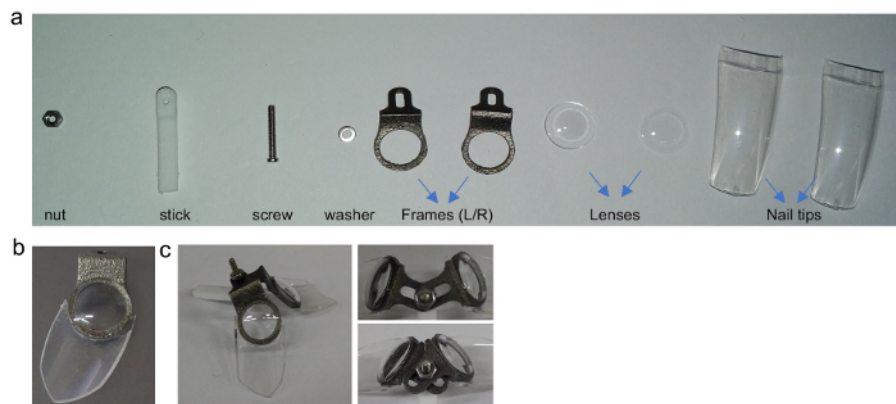
Figure 1: The design of the skull-mounted eyeglasses. (a) All parts needed for assembling the mouse glasses. (b) An example of the position of the frame and the nail tip for the right side of the eye. (c) An example of one set of assembled glasses. Adjust the joint part to change the angle of the frames to fit for mice in different ages. This figure has been modified from Jiang, X. et al 4 , available under a Creative Commons Attribution 4.0 International License. http://creativecommons.org/licenses/by/4.0/ . Please click here to view a larger version of this figure.
