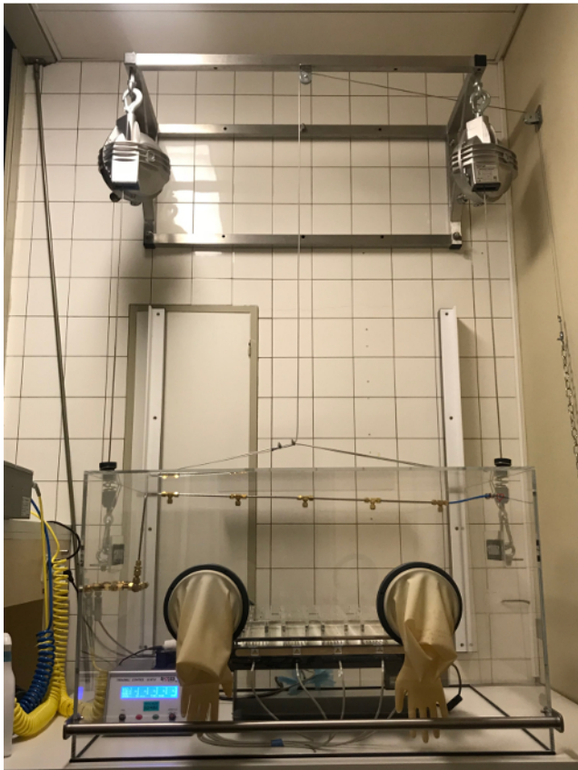
Figure 1: Hypoxic setup. The treadmill is placed inside the homemade glovebox, which is linked to a gas mixer. Please click here to view a larger version of this figure.
