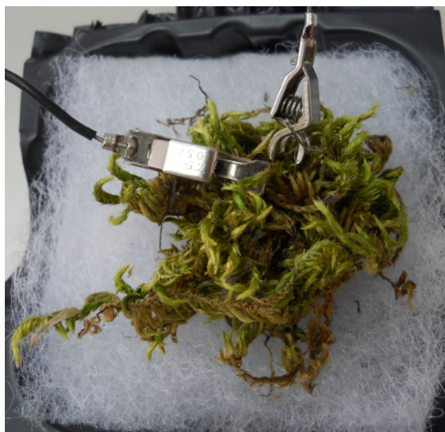
Figure 2: Correct placement of the clips in a moss ( Homalothecium aureum ). The image shows how to place the clips to maintain a minimal distance between the clips without damaging the bryophyte. Please click here to view a larger version of this figure.
