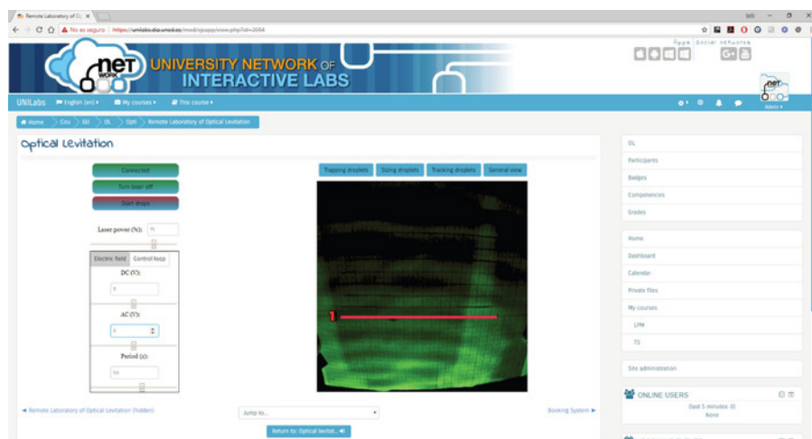
Figure 9: Remote lab interface: sizing a droplet. In remote experimentation, this web application interface is used to determine the size of a trapped droplet. The diffraction pattern displayed by the lab webcam and the scale allow users to determine the size of the trapped droplet. Please click here to view a larger version of this figure.
