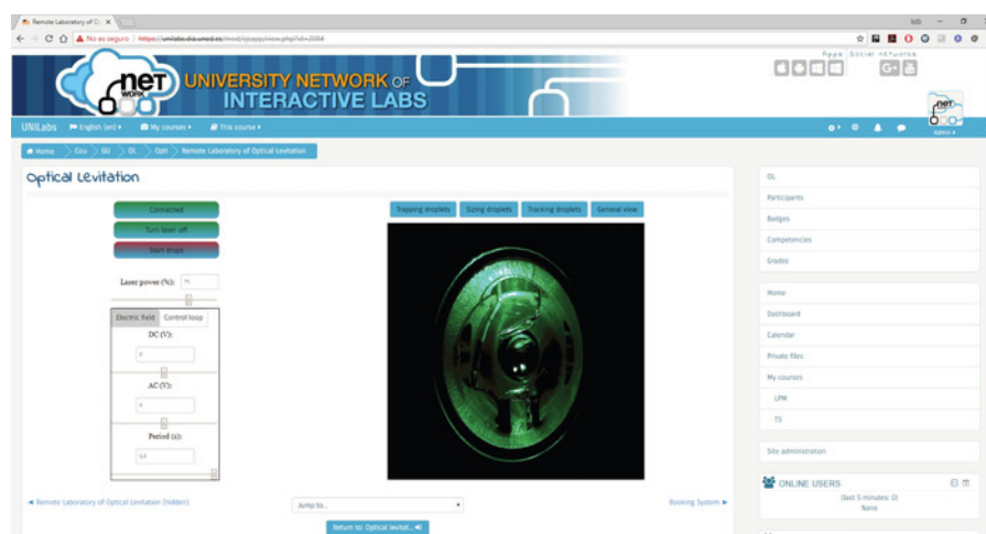
Figure 8: Remote lab interface: trapping a droplet. In remote experimentation, this web application interface is used to trap a droplet. A trapped droplet can be seen in the image provided by the lab webcam due to the scattered light. Please click here to view a larger version of this figure.
