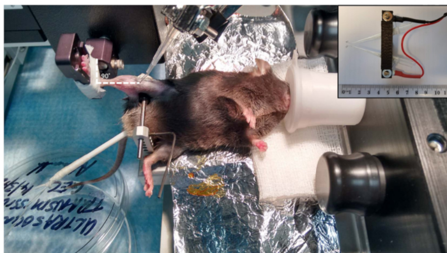
Figure 2: Mouse setup. Overview of the position of the anesthetized animal. The right knee clamp is placed so that the knee is at 90° and so that the foot and the ankle are at 90° angles (dotted white line). Contraction of the dorsiflexors muscles is achieved by stimulation of the peroneal nerve, which is located just under (distal to) the head of the fibula. We use custom-designed electrodes (inset); however, needle electrodes that are provided with the unit, or purchased separately, are also sufficient. Please click here to view a larger version of this figure.
