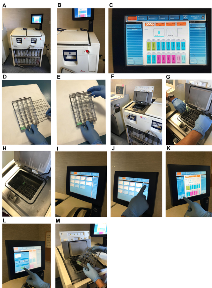
Figure 3: Description of automated processing. (A, B) automated processor. (C) Icon describing the correct paraffin wax melting temperature. (D, E) Insertion of the cassette in the metal basket (D) and its closure (E). (F, G, H) Insertion of the metal basket in the retort. (I, J, K) Selection of the processing protocol. (L) Running of the protocol. (M) Removal of the basket form the retort. Please click here to view a larger version of this figure.
