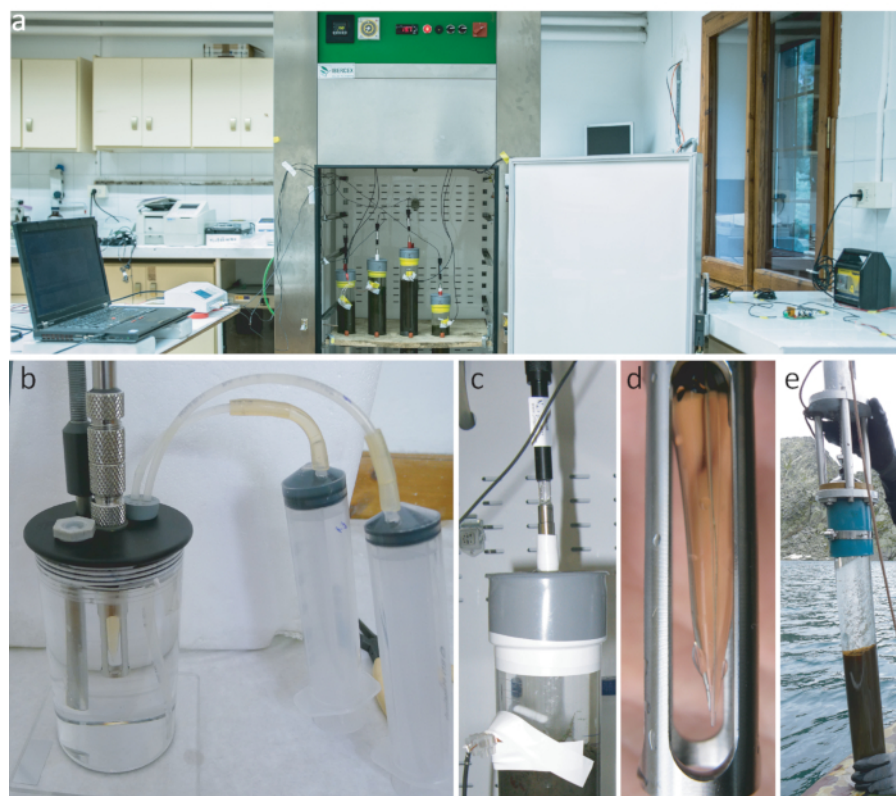
Figure 1: Experimental setup. (a) General experimental setup to estimate sediment denitrification rates using cores and N_2O microsensors. The incubation chamber ensures darkness and controlled-temperature ( \pm 0.3^\circ \text{C} ) conditions. Five intact sediment cores can be processed simultaneously using their respective N_2O sensors. (b) N_2O sensor calibration chamber. We adapted it with rubber stoppers and syringes to mix the N_2O water (see protocol step 3.4.3). There is a thermometer to control the water temperature. (c) Close-up of a sediment core sample with the sensor inserted into the central hole of the PVC cover and the joints sealed with adhesive tape. The stirrer is hanging in the water, and the electromagnet is close to it and fixed to the external part of the acrylic tube. (d) Close-up of the N_2O microsensor tip protected by a metal piece. (e) A sediment core that has just been recovered. It was sampled from a boat in a deep lake; the acrylic tube with the core is still fixed to the messenger-adapted gravity corer 19 . See the Table of Materials for all the items needed to perform this method. Please click here to view a larger version of this figure.
