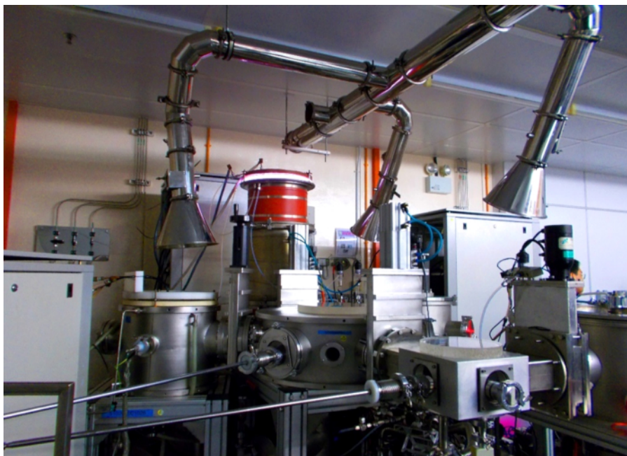
Figure 14: Inductively Coupled Plasma Facility for synthesis of novel materials at the Plasma Sources Application Centre / Space Propulsion Centre, Singapore. A powerful plasma system enables synthesis of silicon-based materials for innovative, highly efficient solar cells, as well as boron nitride and other nanostructured materials for applications in the modern miniaturized thrusters. Please click here to view a larger version of this figure.
