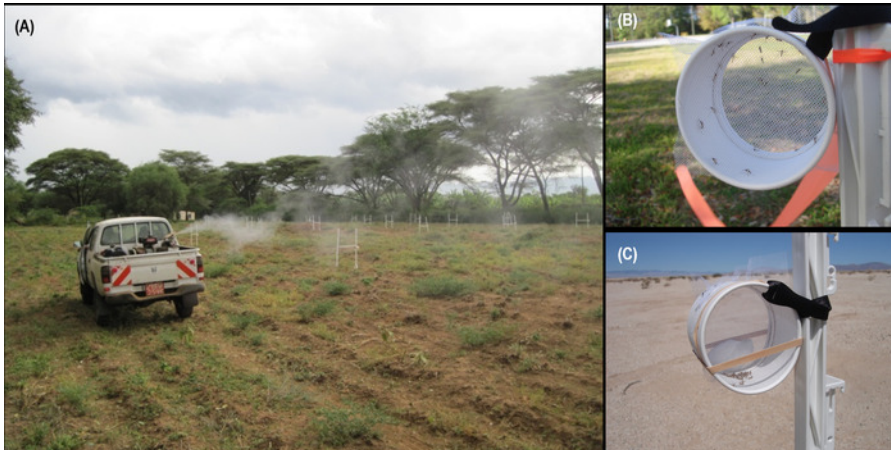
Figure 4: Vehicle mounted thermal fog spraying a grid in warm-arid equatorial location. A truck mounted ULV sprayer driving along a spray line directing pesticide spray through a grid of sentinel cages in an open field (A). Similar to Figure 2 , each sentinel position is fitted with a second pole to support a cotton ribbon to collect pesticide droplets for later analysis with gas chromatograph/mass spectrometry. Close-ups of sentinel cages (B) in a warm temperate environment before spray and (C) in a hot-arid environment after spray. Please click here to view a larger version of this figure.
