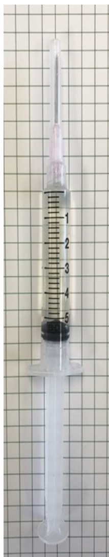
Figure 2: Correctly extracted and sealed extracted pore solution in a 5-mL syringe. The extracted pore solution should appear clear ( i.e. , no visible particles) and should be sealed with no air bubbles within the syringe.
