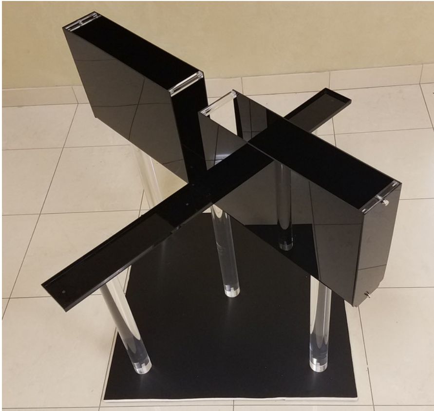
Figure 1: Elevated plus maze (EPM) used for testing rats. Each arm is 10 cm wide and 50 cm long, with two opposite arms opened with a raised edge. The two closed opposite arms are equipped with 30 cm-high walls. The runway height from the floor is 55 cm. Please click here to view a larger version of this figure.
