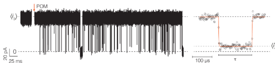
Figure 2: Nanopore-based detection of individual metallo-nanoparticles. An illustration of ionic current time series traces that occur before and after the addition of a POM solution to the nanopore apparatus. The partitioning of individual anionic POMs into the pore causes transient current reductions in the mean open pore current, \langle I_o \rangle . (Right) A typical event, illustrating the mean current of the blockade ( \langle I \rangle ) and the residence time ( \tau ) of the particle in the pore. The applied potential was -120 mV, and the solutions contained 1 M NaCl, 10 mM \text{NaH}_2\text{PO}_4 at pH 5.5. The cis compartment also contained 30 \mu\text{M} of 12-phosphotungstic acid. The current blockade depth ratio ( \langle I \rangle / \langle I_o \rangle ) and the residence times ( \tau ) provide information about which POM species are present in solution. Under the conditions we used here, the \alpha HL channel does not gate (spontaneously close) when POMs are not present. Please click here to view a larger version of this figure.
