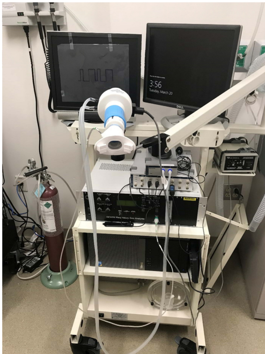
Figure 2. Equipment setup for capnographic measurements. Shown in this figure are the pneumotach and gas analyzer required for capnographic measurements. The left monitor and tracing are used by the participant as a guide in generating the flow pattern while data are observed on the right monitor by the investigator. Please click here to view a larger version of this figure.
