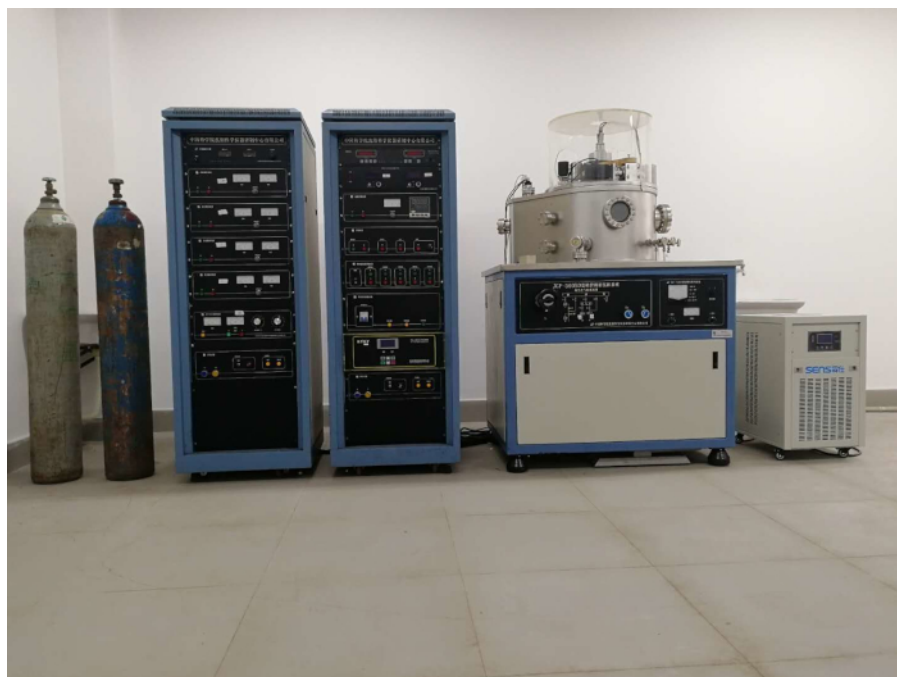
Figure S1: Picture of the RF sputtering system. Please click here to view a larger version of this figure.
