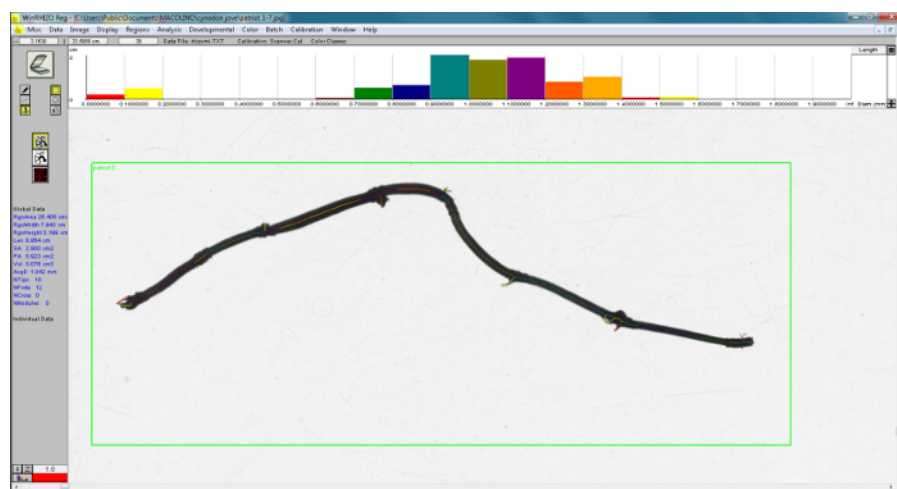
Figure 7: Example layout of digital image analysis from WinRHIZO software. The scanned image in the foreground and the bar charts in the upper part of the screen image show the length distribution in selected diameter classes. The colored lines indicate the image analysis, and each color corresponds to colors of diameter classes reported in the bar charts. Please click here to view a larger version of this figure.
