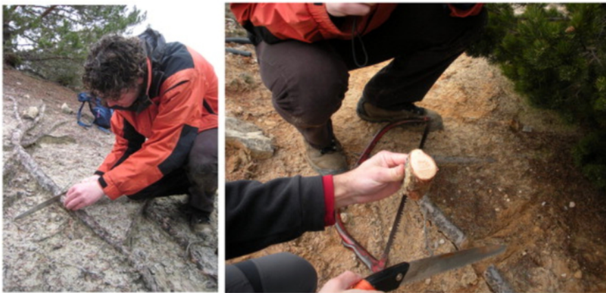
Figure 2: Example of how to conduct field sampling. At least 30 exposed roots are selected and, subsequently, cut with a handsaw. Please click here to view a larger version of this figure.
