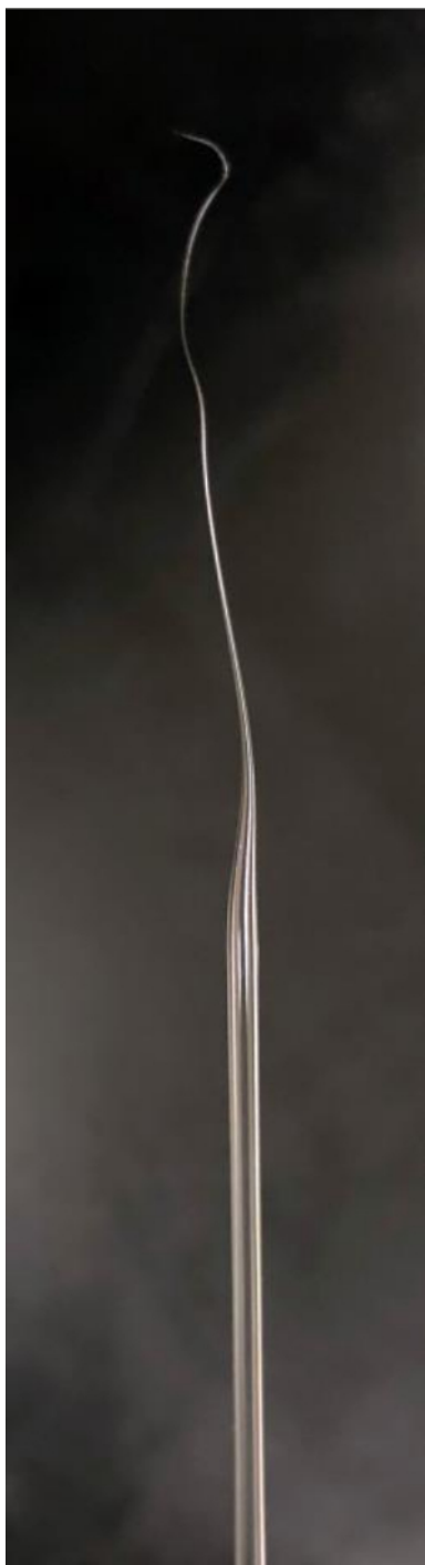
Figure 2: Representative image of the micro cell scraper pulled from a Pasteur pipette. Please click here to view a larger version of this figure.
