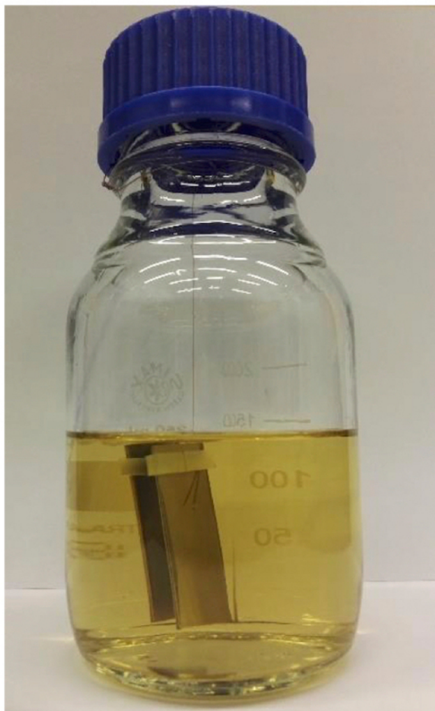
Figure 1: Exposure of mild steel in the aggressive E85 fuel during the static test. Please click here to view a larger version of this figure.
