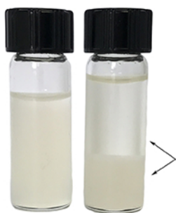
Figure 1. Illustration of congealed (left) and separated (right) water solution test vials. A small test vial should be sampled to assess the viability of the water solution. If the water solution congeals (left), proceed with the next step in the phantom construction protocol. If the water solution separates (indicated by the two arrows on the right vial), the water solution needs to be re-prepared before it can be used for the formation of the phantom emulsion.
