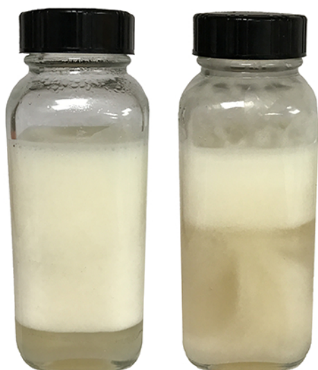
Figure 2. Example of unsuccessful phantom emulsions. Visually inspect the phantom approximately 10 min after pouring to determine if the emulsion will properly set. If the phantom begins to separate ( left ) or appears inhomogeneous ( right ), the phantoms need to be remade.
