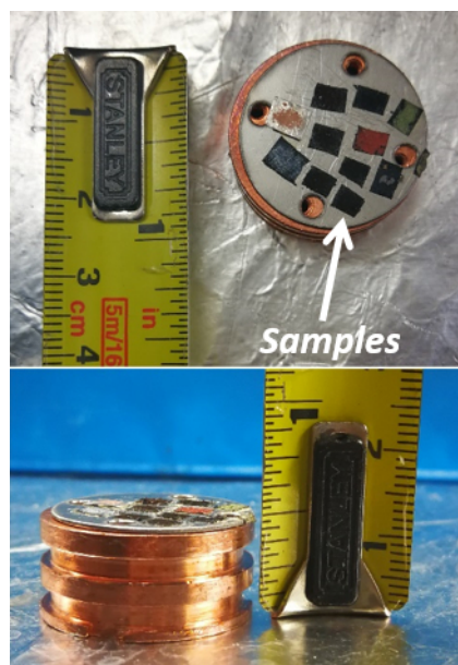
Figure 1: The sample holder and pasted samples. The sample holder is a copper cylinder with a height of 0.5 inches and a diameter of 1.0 inches. The samples are typically several mm in size. Please click here to view a larger version of this figure.
