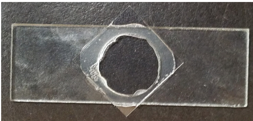
Figure 1: Glassslide with coverslip attached. A 25 mm x 25 mm, flame-treated coverslip is attached to a 75 mm x 25 mm glass slide with a 20 mm in diameter circular hole cut in the center and sealed with vacuum grease. Note the lack of visible bubbles or gaps in the vacuum grease under the coverslip. Please click here to view a larger version of this figure.
