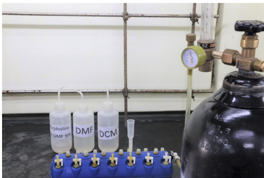
Figure 1: Manual peptide-synthesis apparatus for solid phase peptide synthesis. The columns were placed on the vacuum manifold through the three-way stopcocks and the apparatus was connected to a nitrogen or argon gas line for the bubbling. Please click here to view a larger version of this figure.
