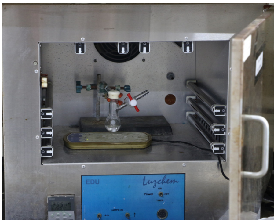
Figure 2: The photoreactor device used for the photoreactions. The device was equipped with ten 350 nm lamps ( Table of Materials ) for UV irradiation and an argon gas tank to ensure that the photoreactor was filled with argon gas prior to and during the photoreactions. Please click here to view a larger version of this figure.
