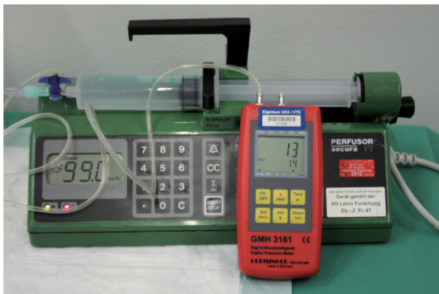
Figure 3: Equipment for burst pressure measurements. Automatic pump (syringe filled with saline) and pressure meter connected via a 3-way-stopcock. Please click here to view a larger version of this figure.
