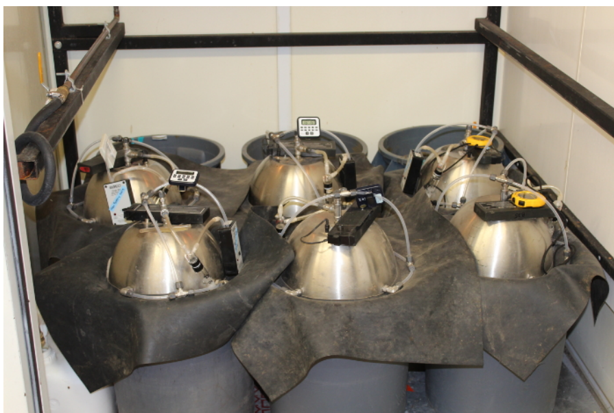
Figure 1. Simulated bedded packs in plastic containers with stainless steel flux chambers and rubber skirts attached and ready for air sampling. The simulated bedded packs are located inside the environmental chambers. Please click here to view a larger version of this figure.
