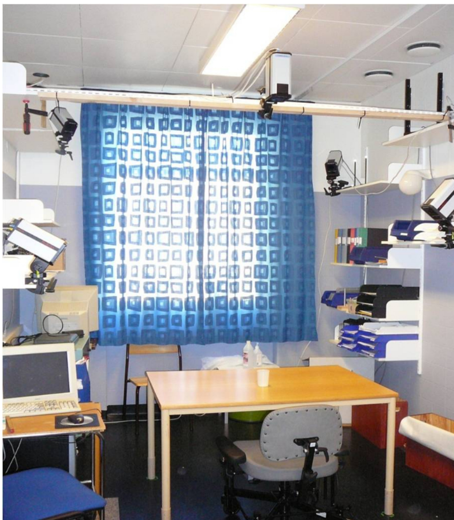
Figure 1: The 5-camera motion capture system set-up for drinking task. From each camera, infra-red light flashes reach retro-reflective markers and reproduce the 2D position of the marker in the cameras image sensor with high spatial resolution and accuracy in real-time. The 3D coordinates of the marker are created when two cameras are viewing the same marker from two different angles. Four cameras are mounted on the walls around the testing area facing slightly downward at approximately 2 m distance and one camera is mounted facing down from the ceiling above the measurement area. Please click here to view a larger version of this figure.
