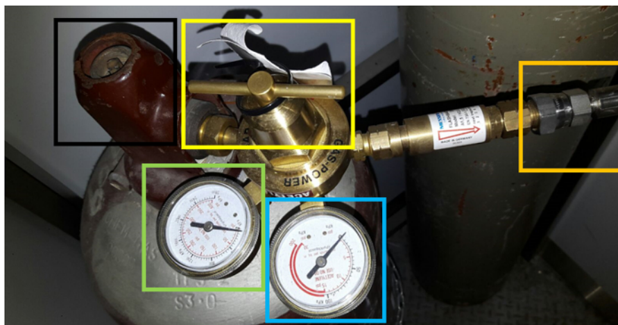
Figure 1: Gas regulator set-up with gas cylinder. A gas regulator is attached to the gas cylinder to regulate the gas pressure pump into the SFMT reactor. The high pressure gauge (green box) is adjusted by attaching a wrench to the part (black box) by turning clockwise or anti-clockwise. The low pressure gauge (blue box) is regulated by the tap valve (yellow box). The arrestor (orange) is connected to prevent any flame from entering the gas cylinder for safety purposes. Please click here to view a larger version of this figure.
