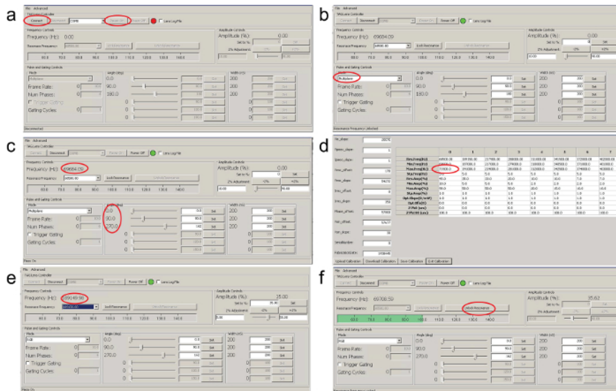
Figure 3. TAG lens software settings. See section 4.2 TAG lens settings for more information. Please click here to view a larger version of this figure.
