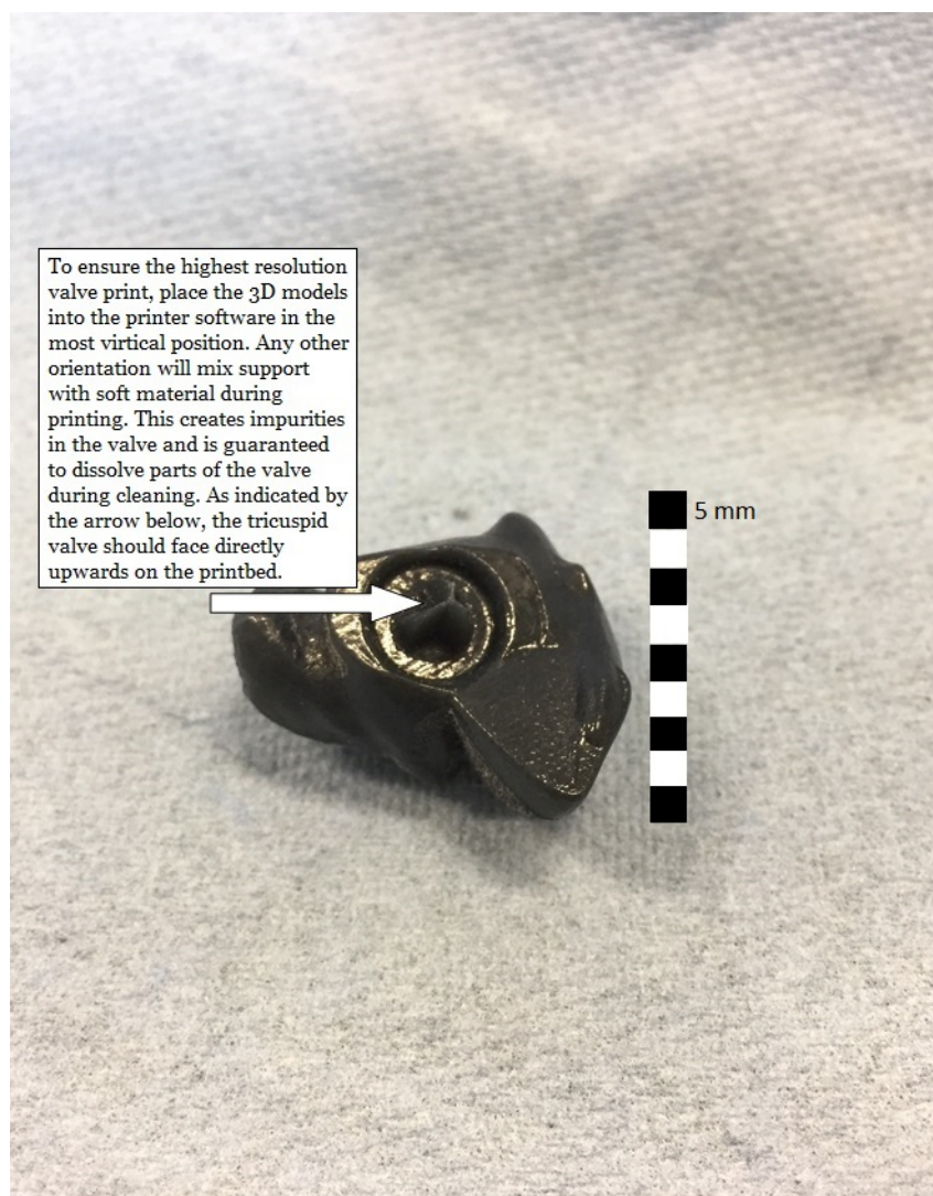
Figure 3: When printing the molds, the heart valve parts should always be printed facing an upward position in the glossy mode to guarantee accurate geometry. This also prevents support material from clogging up the cavities of the valve, which might disrupt the geometry after the cleaning process is complete.
