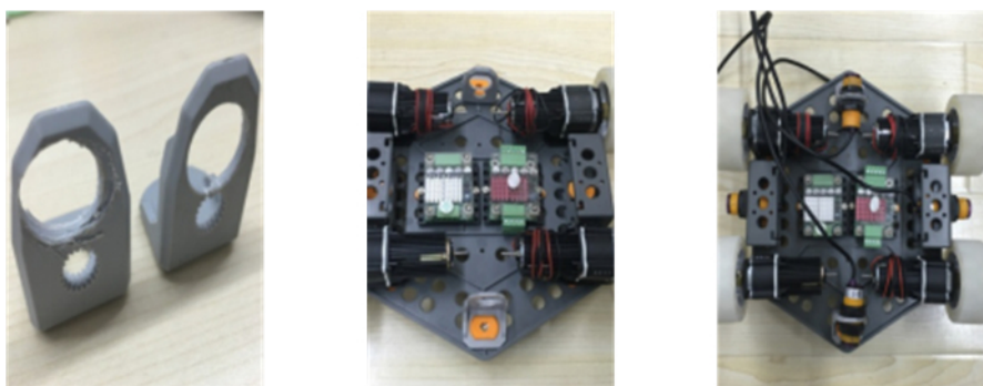
(A) Structural part (B) Install the motor drive underneath the chassis (C) Install the infrared sensor
