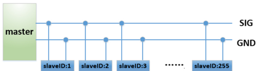
Figure 6: Electrical connection principles. Please click here to view a larger version of this figure.
