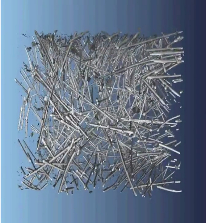
Video 2. Steel fiber distribution of R-0.8% from X-ray computed tomography tests. Results of X-ray computed tomography tests give the spatial distribution of steel fibers in the specimen and prove that the steel fibers in ASFRC specimens are highly aligned while those in SFRC specimens are randomly distributed. Please click here to view this video. (Right-click to download.)
