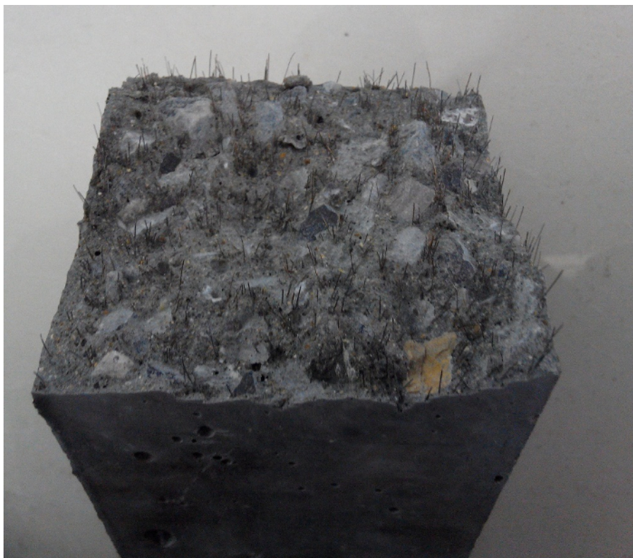
Figure 7. Aligned steel fibers on the fractured section of a steel fiber reinforced concrete sample. Although a number of coarse aggregates exist, the steel fibers in concrete are still effectively aligned. Please click here to view a larger version of this figure.
