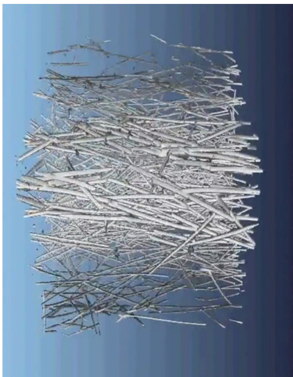
Video 1. Steel fiber distribution of A-0.8% from X-ray computed tomography tests. Results of X-ray computed tomography tests give the spatial distribution of steel fibers in the specimen and prove that the steel fibers in ASFRC specimens are highly aligned. Please click here to view this video. (Right-click to download.)
