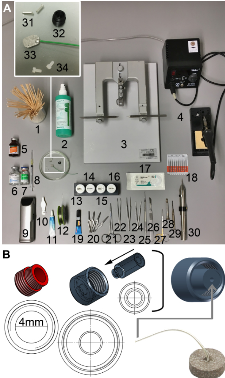
Figure 1: Supplies for surgery and technical scheme of the tES socket and electrode cap unit. (A) 1. Cotton swabs, 2. disinfectant, 3. stereotactic frame, 4. soldering iron, 5. analgesic (e.g., carprofen), 6. & 7. anesthetics (e.g., xylazine & ketamine), 8. syringe, 9. clipper, 10. ear puncher, 11. eye ointment (e.g., bepanthene), 12. lead-free tin-solder, 13. two-component dental acrylic cement (DAC), 14. iodine, 15. 3% H 2 O 2 , 16. 0.9% saline, 17. synthetic braided non-absorbable suture (e.g., Mersilene 4-0), 18. drill bits, 19. cyanoacrylic glue, 20. bulldog clamps 21. homeostatic forceps, 22. bent, serrated tip forceps, 23. straight, sharp tip forceps, 24. straight, tissue forceps, 25. dental spatula, 26. scalpel, 27. scissors, 28. hand drill, 29. screw driver, 30. motor driven drill, 31. female connectors, 32. tES socket, 33. square platinum electrode attached to cable, soldering joint covered with histoacrylic glue, 34. plastic screws. (B) tES socket (red) for fixation on the rodent skull with an inner diameter of 4 mm; the electrode unit (grey) is built by a screw cap and an inner stamp with a center hole leaving room for the cable of the Ag/Cl disc electrode, which is glued to the bottom of the stamp. This allows for maximal stability of the set-up and avoidance of wire breaks at the sensitive wire-electrode-connection point. Please click here to view a larger version of this figure.
