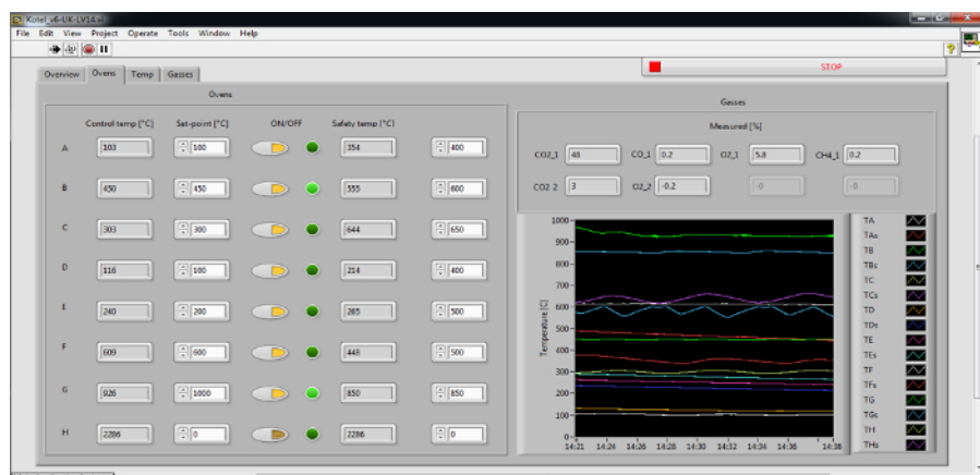
Figure 2: Screenshot of temperature data acquisition for the preheating system. Please click here to view a larger version of this figure.
