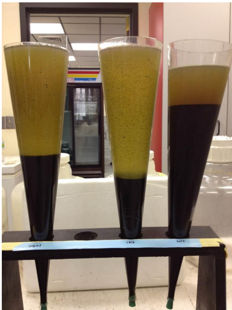
Figure 3: Imhoff settling cones used to collect the suspended particulates captured in the settling tank. Please click here to view a larger version of this figure.
