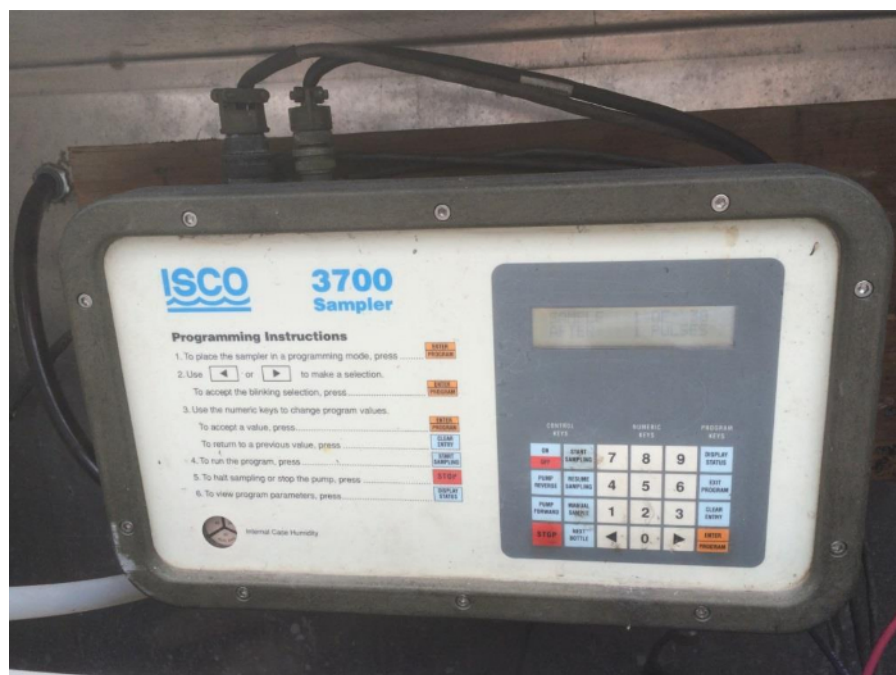
Figure 1: ISCO sampler used to program auto-sampling procedures for the composite drainage water and the particulates water sampling. Please click here to view a larger version of this figure.
