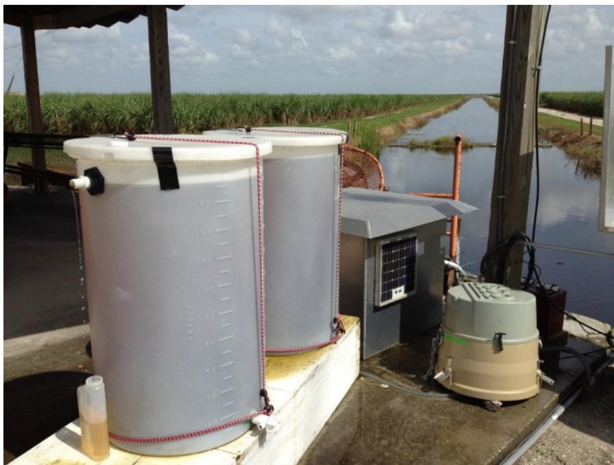
Figure 2: Two 200 L tanks used to collect drainage water. Suspended particulates settle out at the bottom of the tank and are transferred in five-gallon buckets. Please click here to view a larger version of this figure.
