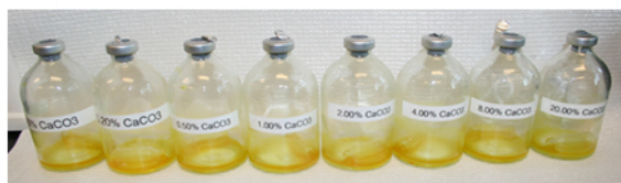
Figure 10. \text{CaCO}_3 Measurement. (a) A standard curve for \text{CaCO}_3 is created using the voltage readings from the pressure transducer based on known percentages of \text{CaCO}_3 (b) mixed with powder glass beads or sand.
