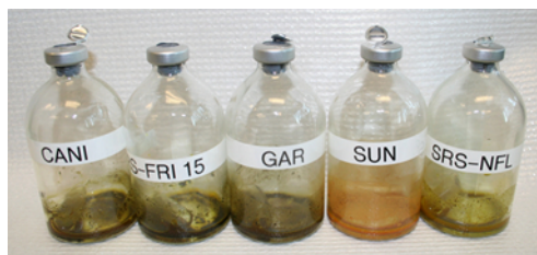
Figure 9. Reaction Vessels for the Modified Pressure-calcimeter Method. Reaction vessels for the modified pressure-calcimeter method are serum bottles containing a 0.5 dram vial with 2 mL acid reagent and a 1 g soil sample.
