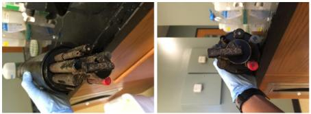
Figure 7. Images Showing the Fouling on the Sensor Surfaces (left) and Clean Sensing Surfaces of the Sensors (right) after Wiping with a Brush and Wiper. Please click here to view a larger version of this figure.
