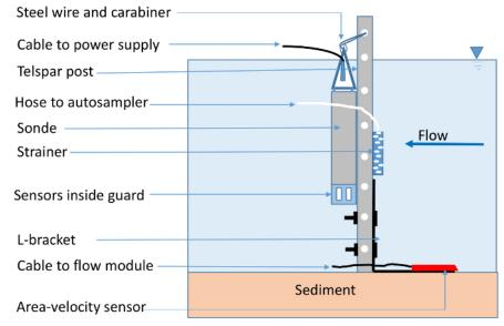
Figure 1. Layout of a Typical Instream Monitoring Station (Not to a Scale).
