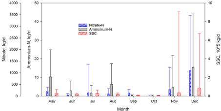
Figure 4. Monthly Variation of Nitrate, Ammonium, and SSC Load (kg/d) at the Outlet of the Little River Ditches Basin. The values are median ± interquartile range. Please click here to view a larger version of this figure.
