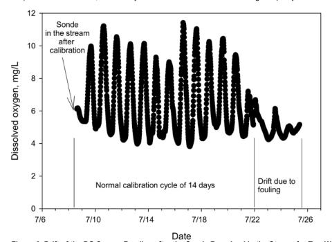
Figure 6. Drift of the DO Sensor Reading after the Sonde Remained in the Stream for Two Weeks.
