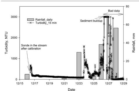
Figure 8. Turbidity (NTU) in the Stream Before and After Sediment Buildup in the Sonde Guard.
