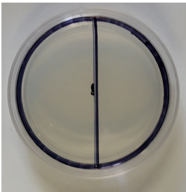
Figure 1: A Visual Representation of Markings to Indicate Copper Solution Placement on the Underside of a 5 cm Petri Dish. These indications are used to ensure that the sections of the plate have been appropriately measured and serve as a guideline when transferring the bacterial patch and then copper solution onto the agar surface. Please click here to view a larger version of this figure.
