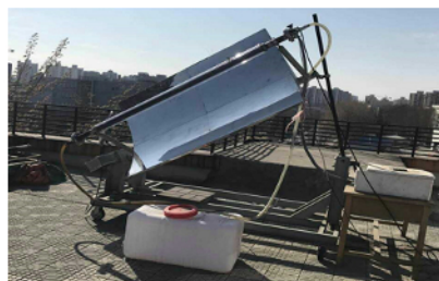
Figure 1: Experimental system for solar adsorption refrigeration. (Top) Schematic of the system; (bottom) Photograph of the experimental setup. The top panel presents the components of the experimental system, which involves the evaporator, the condenser, the vacuum pump, etc. The bottom panel displays the photograph of the assembled adsorption refrigeration system. In the system, the evaporator and the condenser is of the fin-tube structure, a kind of compact heat exchanger. The adsorption bed is reformed from a vacuum solar collector, which can capture solar energy effectively. Please click here to view a larger version of this figure.
