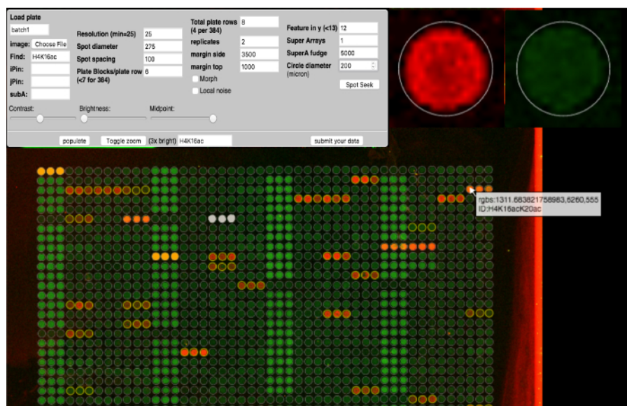
Figure 4: ArrayNinja Analysis Module. A screen shot of the ArrayNinja analysis module is shown. The control panel (top left) shows all of the parameters that can be adjusted to visualize the array, find spots, and align a grid over the array image. Hovering the mouse over a feature shows a zoomed-in view (top right) and displays a popup that contains the identification information associated with that feature (bottom). Reference spots selected for background correction are orange. Features to be excluded from downstream analysis are white. ArrayNinja contains a text-based search feature that highlights matching features in yellow, as shown in the example for H4K16. Please click here to view a larger version of this figure.
