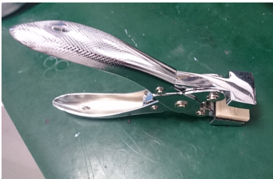
Figure 5: Picture of the special hole punch. The special punching tool is customized for cutting the cavity on the chamber plate. Please click here to view a larger version of this figure.
