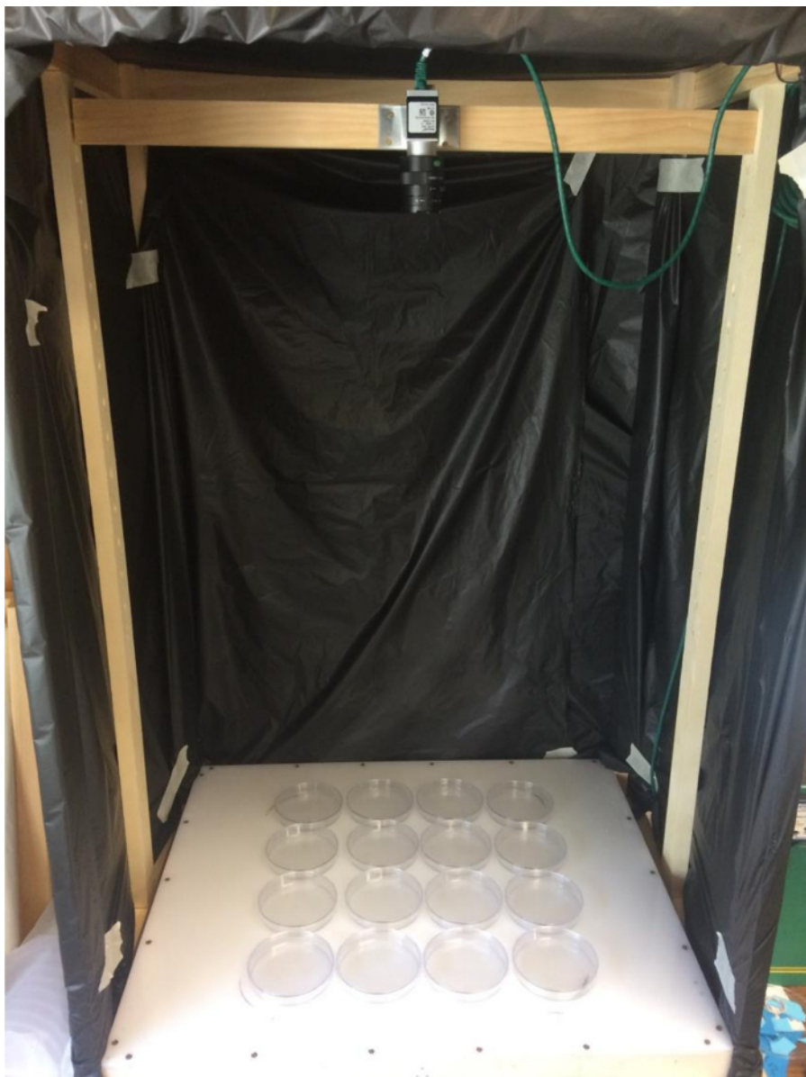
Figure 1: Petri dish arrangement on the light box. Petri dishes are arranged in a 4 x 4 block on top of the light box. This arrangement provides easy identification of the control and repellent treatments for the visual tracking protocol. Please click here to view a larger version of this figure.
