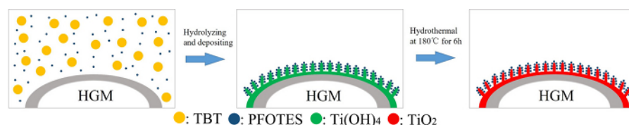
Figure 1: The synthesis scheme of MCHGM. For other samples, such as F-SCHGM and Ti-SCHGM, the processes are quite similar, but without related raw materials. Please click here to view a larger version of this figure.
