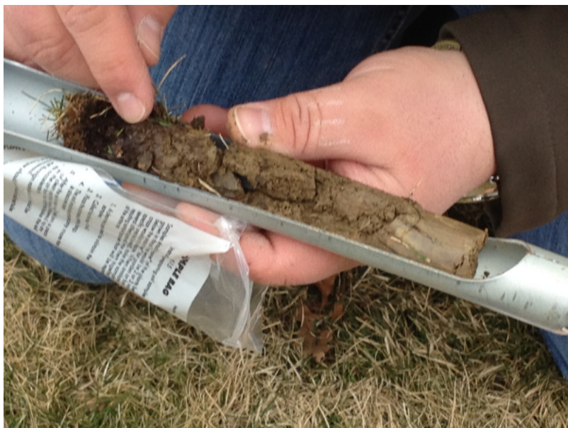
Figure 2. Contaminated soil collected using a soil sampler.
