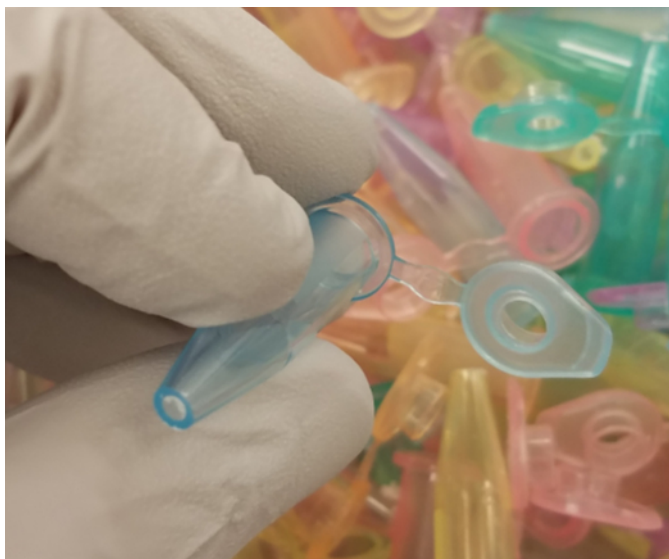
Figure 1. Modified Centrifuge Tube. Modified 0.5 mL microcentrifuge tube with holes in the bottom and top. Please click here to view a larger version of this figure.
