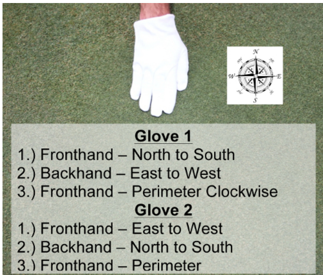
Figure 2: Hand wiping directions. Progression is intended to contact maximum unique treated vegetation surface area to glove. Two gloves are required to avoid overloading cotton when sampling <415 \text{ cm}^2 area; however, this should be confirmed in pesticide- and site-specific conditions prior to experiment initiation. Please click here to view a larger version of this figure.
