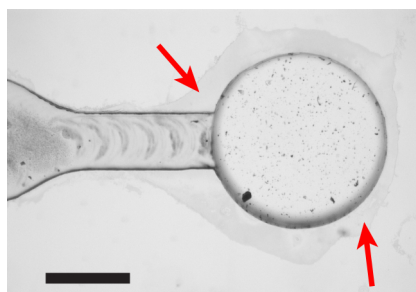
Figure 4: Non-destructive Inspection via Microscopy. Careful inspection with an optical microscope can identify regions of unbonded plastic, particularly near microfeature edges, or on small bonding areas. Unbonded regions (red arrows) appear slightly darker than bonded regions due to the thin air gap between the plastic layers, and colored interference fringes are sometimes also visible in these areas. Identifying regions of poor bonding can indicate the need for a second iteration of bonding, with solvent locally added to trouble spots. Scale bar = 1 mm.
